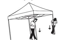
6 Click the Side Tensioning straps on the inside of the canopy onto the frame struts to ensure the overhang / valance is secured and tensioned correctly.
