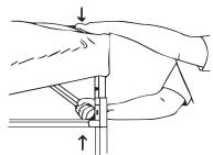
Lift two adjacent outer legs up and pull out the inner legs until they click into your desired height. We recommend extending the legs to the 3rd or 4th hole. You will need to ensure your marquee is secured by using the supplied pegs or ask about our leg weight accessories.
