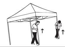
Release auto slider at each corner by pushing the snap button. Repeat on all four corners.
