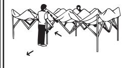
4 Go to each corner of the frame and engage the auto slider by pushing up with one hand while holding down the top of the leg with the other hand. This should then click into place. Repeat on all other legs.
