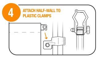
Take the assembled half-wall (A,B,E) and lift above the Plastic Clamps (C,D).
