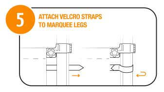
Pull each of the 3 x Velcro Straps (F) straight, and wrap them around the marquee leg, attaching the strap back to itself at the base. Repeat for the other side of the half-wall.
