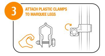
Unwind the nut on Plastic Clamp (C) until the clamp comes apart. Attach clamp to the marquee leg. Screw back together and fasten tightly. Repeat on other leg for Plastic Clamp (D).
