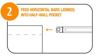
Face the 'hooks' of the joined Horizonal Bars (A,B) down, then feed through the pocket at the top of the Half Wall Fabric Panel (E).
